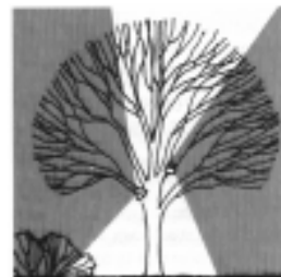
UP AND DOWN LIGHTS PLACED IN TREES
