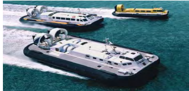
Hovercraft are best suited for shallow areas requiring higher speeds. Recent improvements have reduced their noise impacts.
