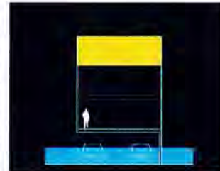
Figure 6. Floodplain management strategies may include floodable first floors and locating critical equipment on the 2nd or 3rd floors.
