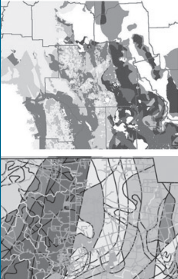
Figure 2.6. These DRASTIC maps of the north central Florida region (top) and Wakulla Springs (bottom) reflect the aquifer's relative vulnerability to pollution. The darker the color, the higher the relative vulnerability.
